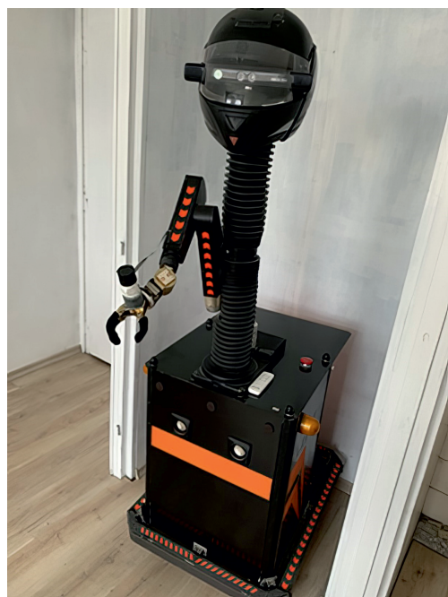
Fig. 2. Robot “AnRI-1” with anthropomorphic manipulator
