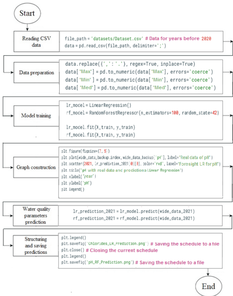
Fig. 2. Machine learning algorithm for predicting aquatic environment parameters
